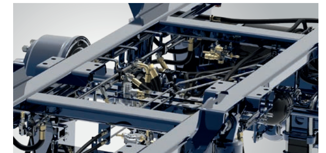
Parallel cross member: > optimised for tippers
